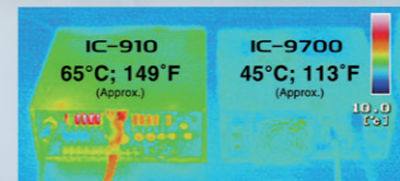
This is a comparison between two transceivers' rear chassis temperatures when continuously transmitting for 15 minutes. The IC-910* rises to 65 °C while the IC-9700 rises only to 45 °C. * Japanese version example when testing at 50 W.
